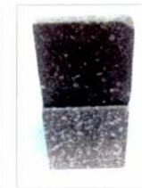
I PODIUM WALLS CONCRETE BLOCK
